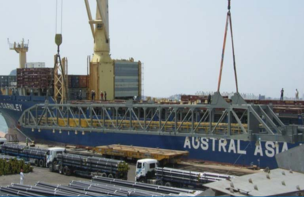
▲ Ship loading : B/W BOOM (Weight : About 120ton)
