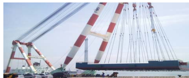
▲ Offloading the pontoon and launching (Sama No. 2200 F/C Offloading and launching operation)
