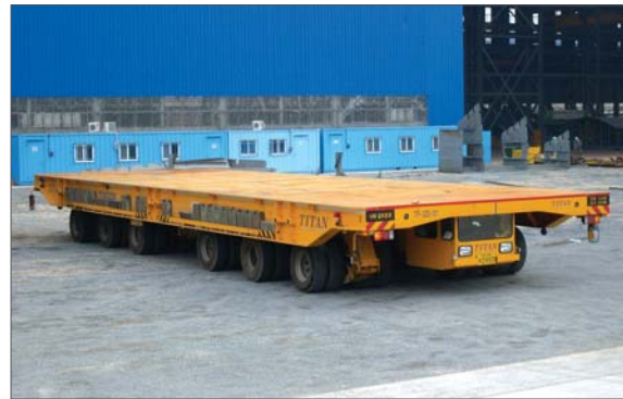
▶ 320ton transporter / 6m(W) x 18(L) _ 2 units
